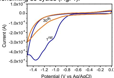
**Figura 1.** Cyclic voltammograms depicting electrochemical reduction (1<sup>st</sup> cycle and 30<sup>th</sup> cycle) of GO on a GCE in 0.10 mol L<sup>-1</sup> acetate buffer electrolyte solution, pH 4.7 at 50 mV s<sup>-1</sup>.
