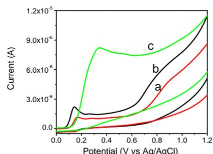
**Figura 2.** Cyclic voltammograms of quercetin (0.18 mmol/L) + naringenin (0.18 mmol/L) obtained in phosphate buffer solution, pH 6.5 and DMSO (1:1) with bare GCE (a) and rGO modified electrode (b) at 25 mV s<sup>-1</sup>, and of the plant extract (c).
